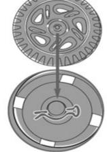
Step 4. Line up each of the tabs in the hub cap with the slots in the wheel, snap hub cap into place.
